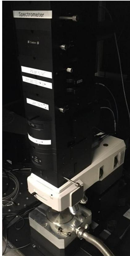
Figure 10: The experimental setup for the advanced practical training (WITec, alpha 300 R).
