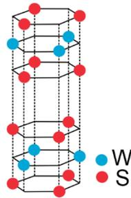
Figure 5: Repeating structure of two-layer units in 2H-stacked WS<sub>2</sub>.
