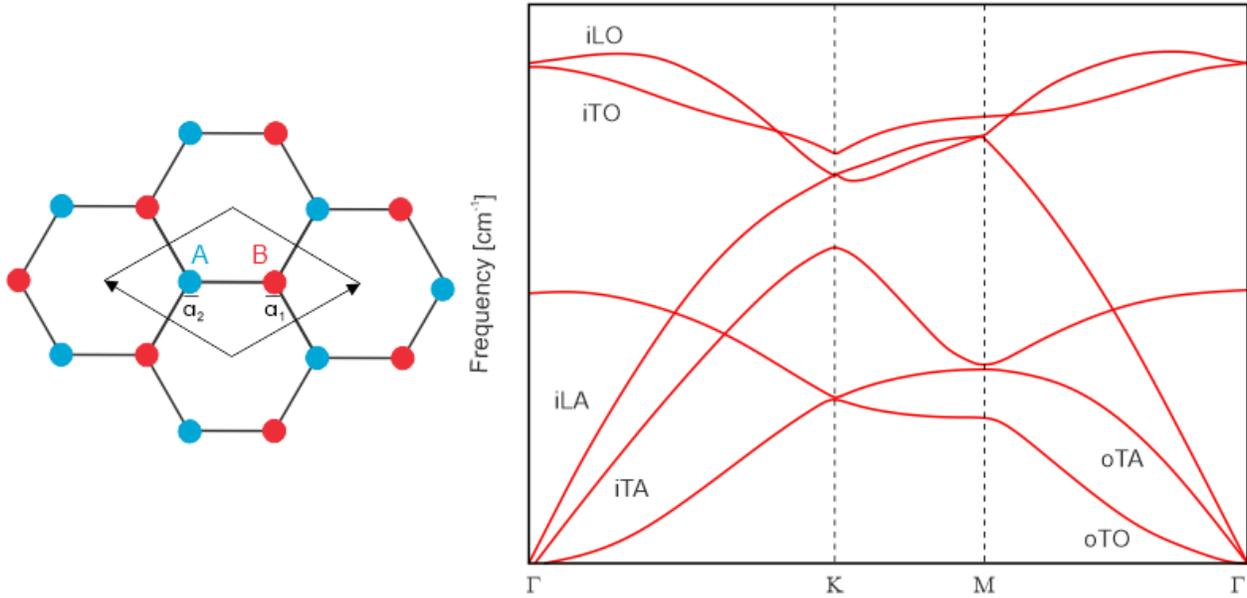
Figure 2: Top view of the real space unit cell of monolayer graphene. The unit cell contains the two inequivalent atoms A and B. Further, the calculated phonon dispersion relation of graphene is shown in reciprocal space (adapted from <sup>4</sup>). The high symmetry points of the Brillouin zone are labelled as K, M and  $\Gamma$ .
