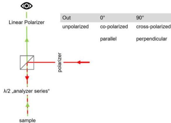
Figure 11: Schematic of the WITec setup for SHG measurements.
