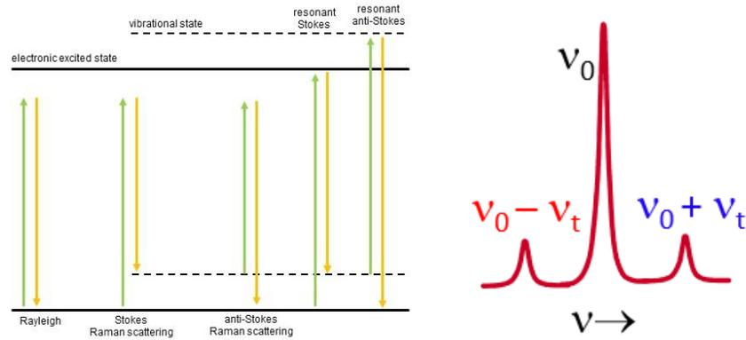
Figure 1: Left: Principles of Raman spectroscopy in a so-called Jablonski diagram. Stokes scattering correlates to an energy decrease, Anti-Stokes scattering correlates to an energy increase. Right: As a function of light frequency, Stokes and Anti-Stokes signals can be detected as satellites right and left of the Rayleigh peak ( $0 \text{ cm}^{-1}$ ), respectively.
